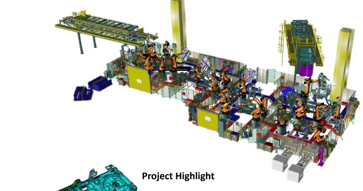
The largest automation project in the history of the company. We have built up joining lines for the complete underbody of new SUV models of SKODA and SEAT.
